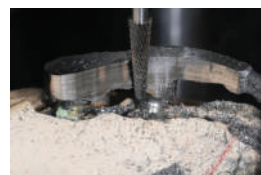
Bar Milling after Casting
